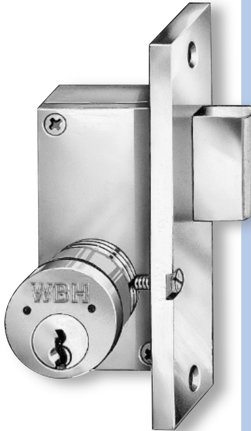
9/08261, LH Lock illustrated. Cylinder is fitted into the body and secured by screw shown.
