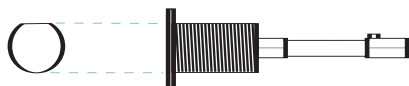
Detail to show 'D' piercing & spindle with spring 'pip' for knob retention
